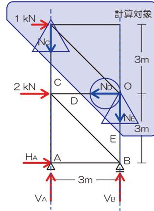
$$\begin{aligned} \sum X &= +1 - N_D = 0 \\ -N_D &= -1 \\ N_D &= 1[kN] \end{aligned}$$
