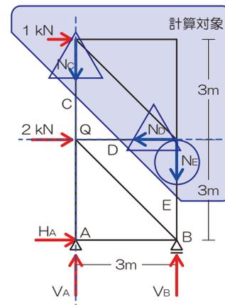
$$\begin{aligned} M_Q &= +N_E \times 3 + 1 \times 3 = 0 \\ 3N_E &= -1 \times 3 \\ N_E &= \frac{-1 \times 3}{3} \\ N_E &= -1[kN] \end{aligned}$$
