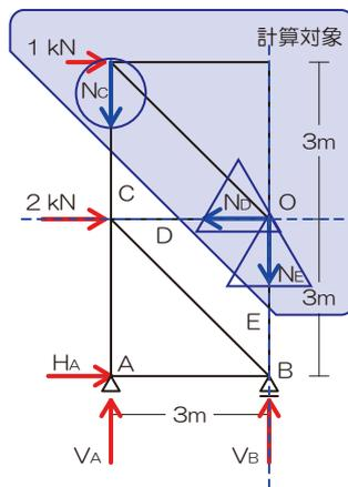
$$\begin{aligned} M_O &= +1 \times 3 - N_C \times 3 = 0 \\ -3N_C &= -1 \times 3 \\ N_C &= \frac{-1 \times 3}{-3} \\ N_C &= 1[kN] \end{aligned}$$
